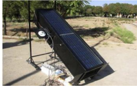
Fig. 2.20 An air-based PVT collector enhanced by aluminium sheets in the air channel (Shahsavari and Ameri 2010).
