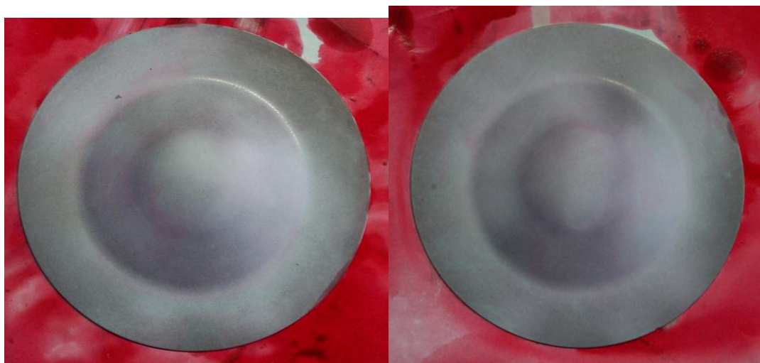
Figure 11: Images from dome testing, after dye penetration testing, of enriched copper UCS steel.
