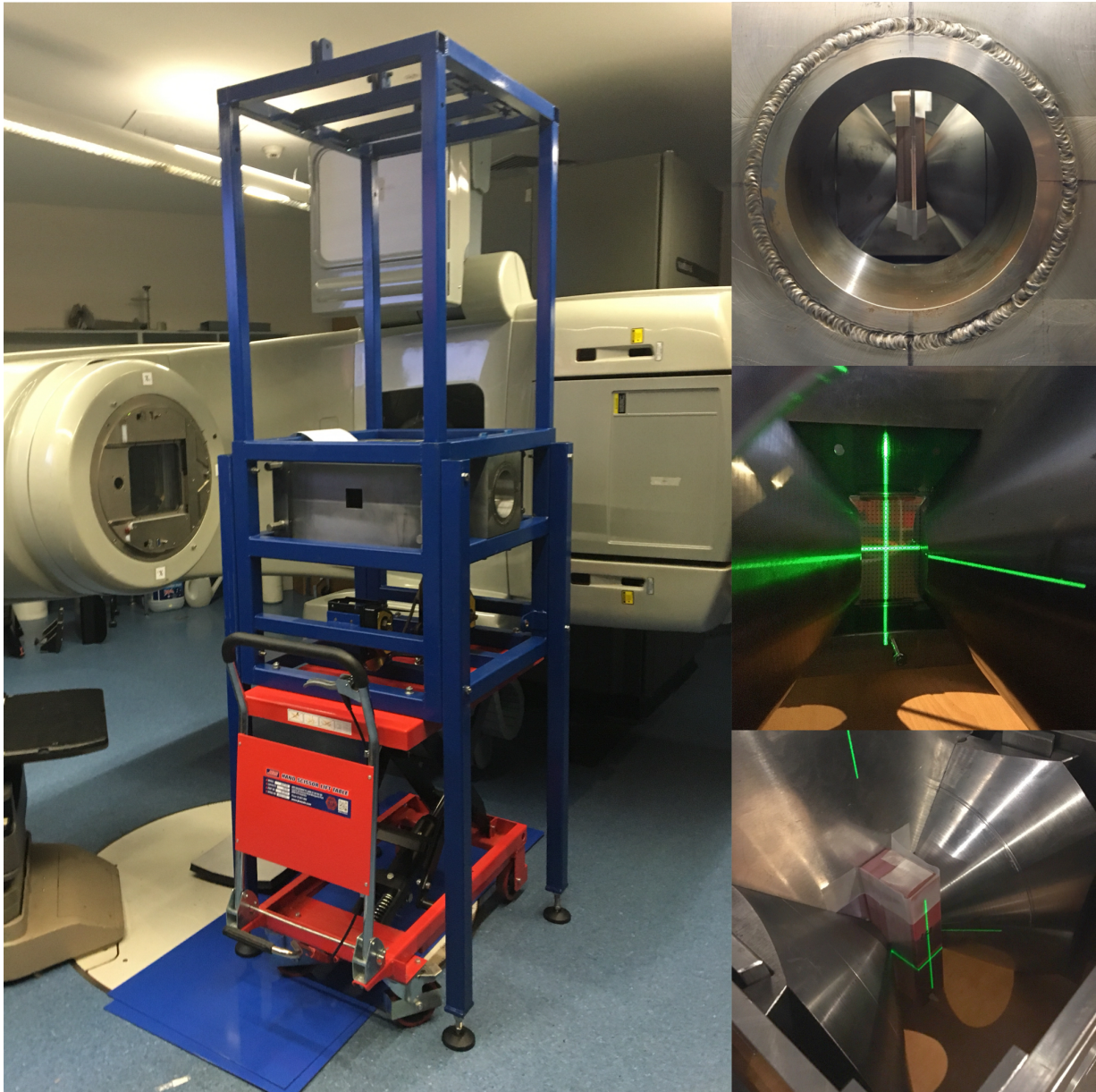
Figure 6.4: Experimental setup. The left image shows the MARDOS device positioned along the central beam axis of a clinical linear accelerator, with the magnet's isocentre at 150 cm SAD. The top right image shows the M512 in a solid water phantom (1.7 cm buildup and backscatter) positioned between the focusing cones of MARDOS, in the inline orientation, within the 0.95 T magnetic field. The middle right figure shows the M512 positioned within slots machined in the focusing cones, in the perpendicular orientation in a 1.2 T magnetic field. The bottom right image also shows the M512 in the perpendicular setup, within the solid water phantom (5cm buildup and backscatter).
