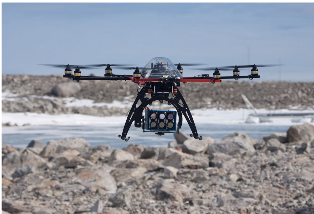
Figure 2 - Oktokopter fitted with Tetracam mini-MCA 6 band multispectral camera
