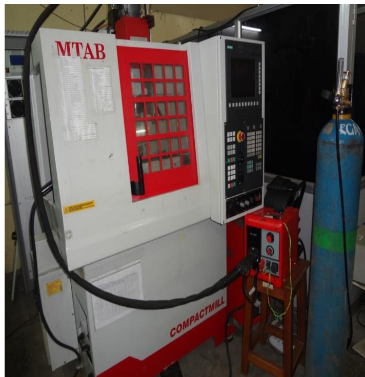
Fig 4.1: CNC machine used for additive manufacturing of the product
