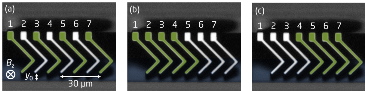
Figure 2: The three sub-probes on an M7PP used for multiplexing during measurements; a) 1357 (20 \mu\text{m} pitch), b) 1234 and c) 4567 (10 \mu\text{m} pitch). The electrode pins used in a given sub-probe are marked with green. The sample itself is highlighted in blue. The direction of magnetic flux density B_z , which is pointing into the sample, is also indicated.
