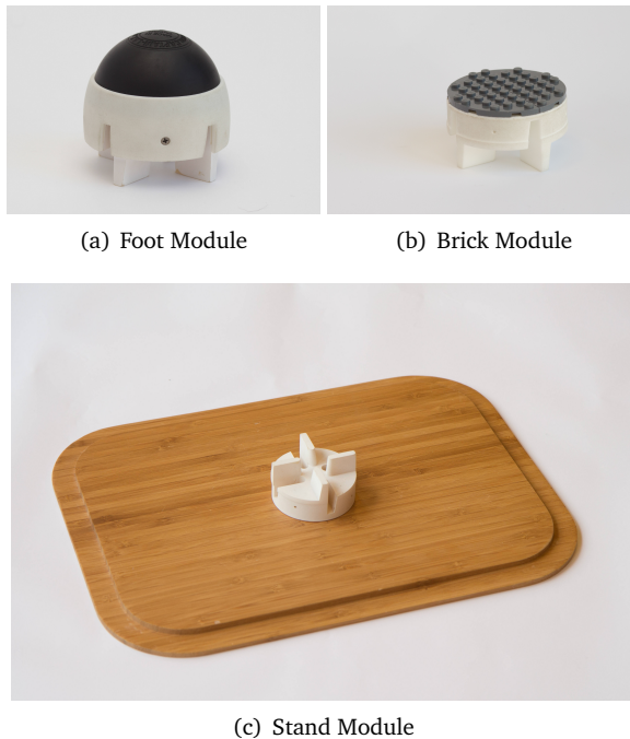
Figure 5.10: Passive Modules can help give extra features and functionality to robotic constructions.
