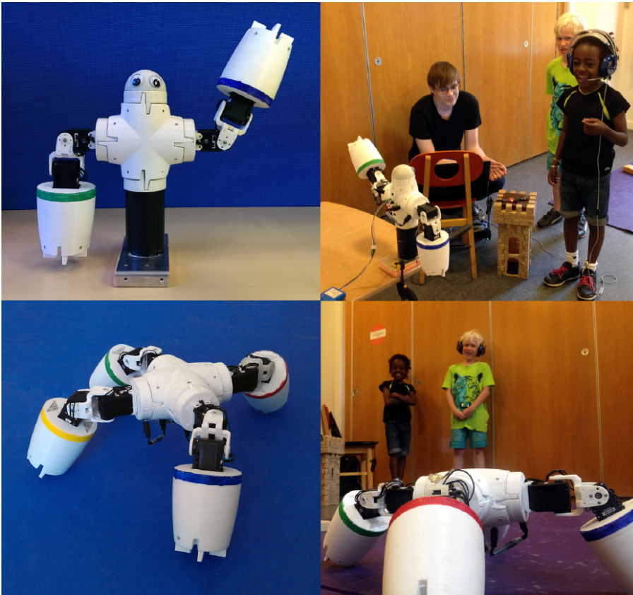
Figure C.1: User testing with two Fable robots controlled using the voice sensor (voice energy and F_0 sensing). The humanoid has controllable arms and the quadruped has controllable locomotion.
