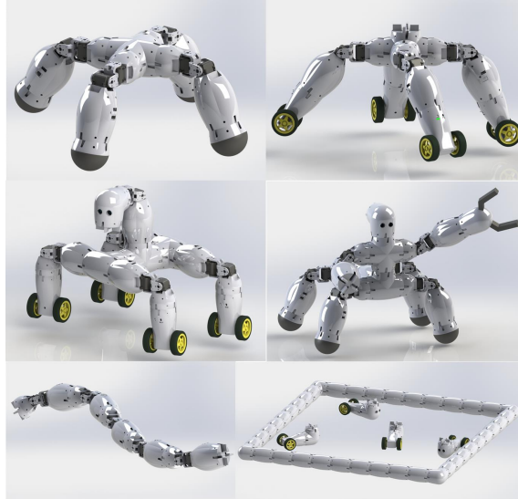
Figure 5.11: A variety of robot assemblies with Fable's library of modules.
