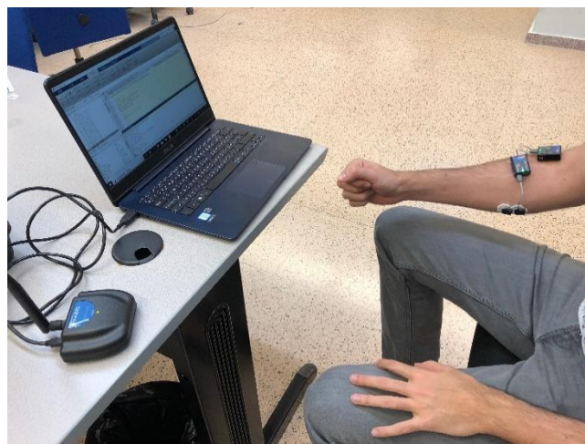
Figure 2. Surface electromyography (sEMG) system acquiring data from a subject.
