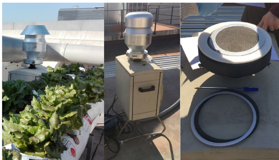
Fig. 2. Example of the experimental design. Left: Image from the periurban rooftop during the first test. Middle: high volume sensor. Right: glass microfibre filters after 48 h of sampling.
