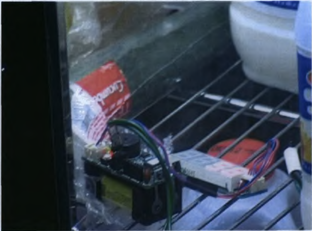
Figure 5-5: A cricket recording the temperature level in the fridge
