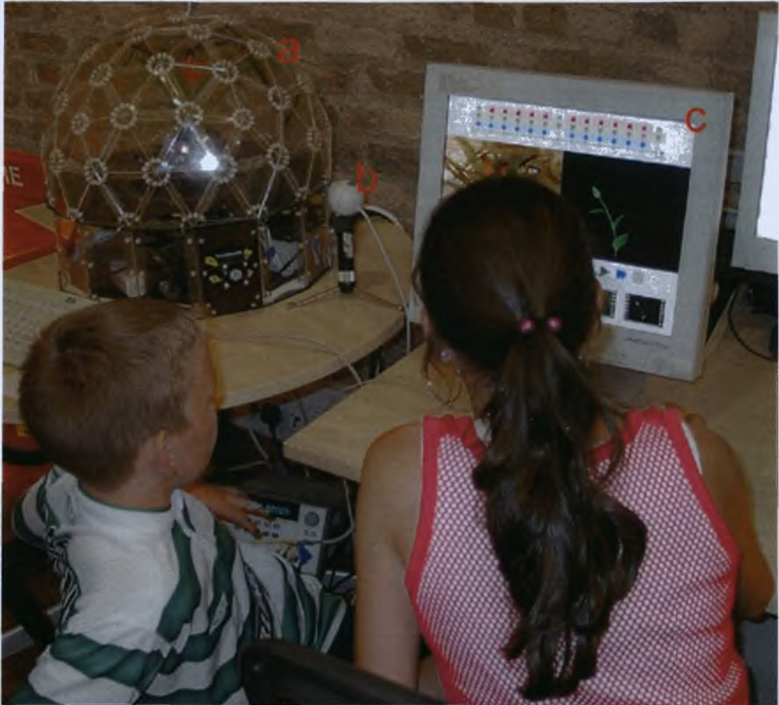
Figure 1-1: The Biosphera platform configuration. (a) dome/terrarium which can host an actual plant, (b) a webcam which record a time-lapse video of the growth of the plant, (c) PC running the Biosphera software with the simulated plant
