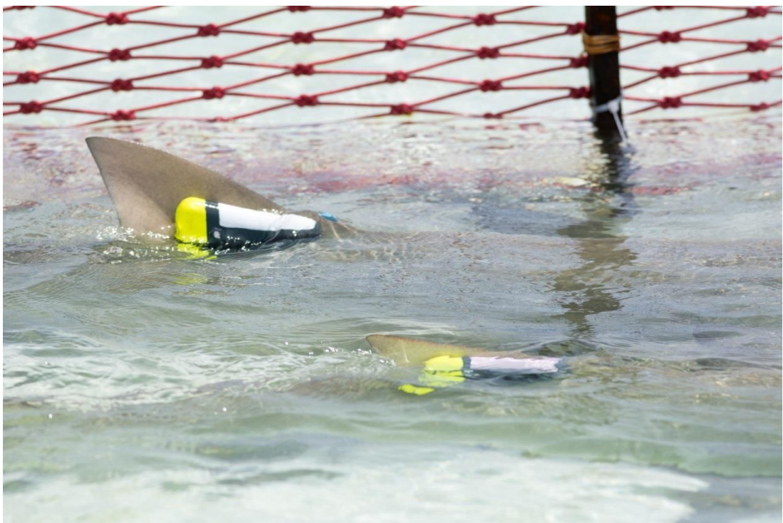
Figure 3.4 CATS Diary tag packages were attached to the first dorsal fin of subadult sicklefin lemon sharks ( N. acutidens ).
