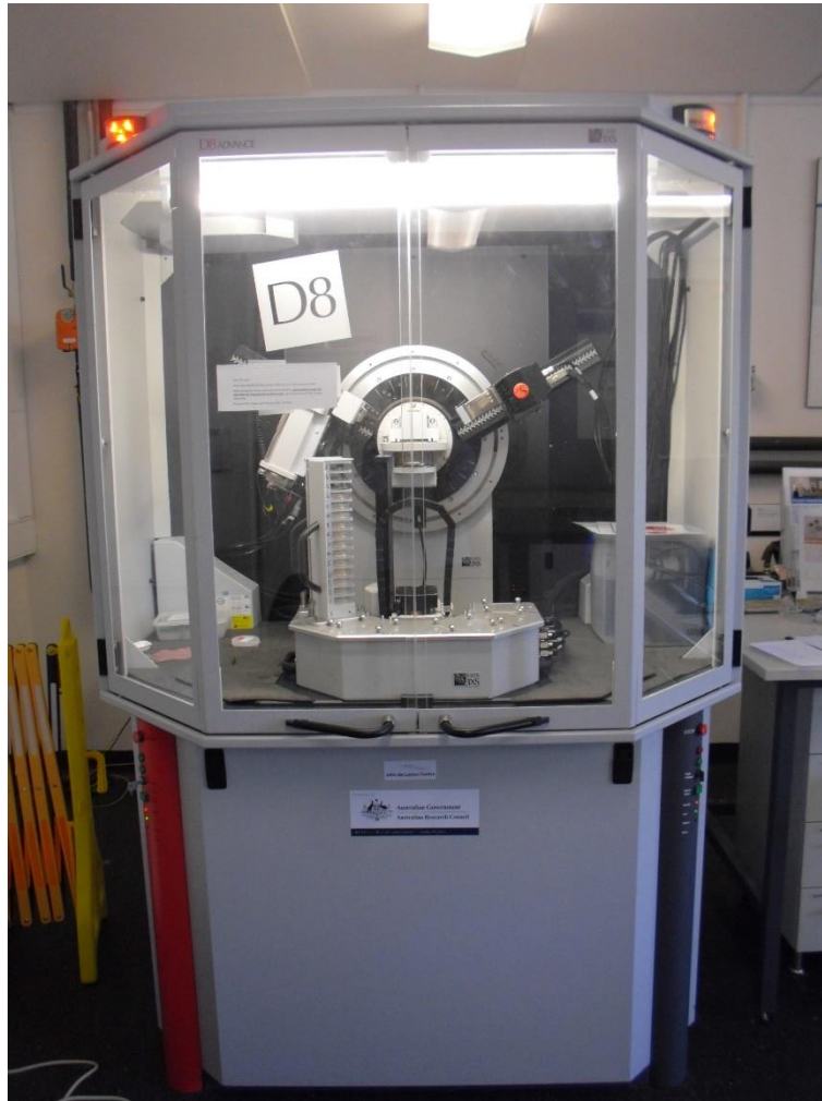
Figure 2. Powder diffraction X-ray diffraction (XRD), Bruker AXS D8 Advance.
