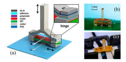
**Figure 1.** (a) Schematic diagram of a motion-amplifying actuator. The system comprises an in-plane extensional lead zirconate titanate (PZT) actuator with a laminated, micro-fabricated half-scissor amplifier to convert small in-plane motions into out-of-plane motions 6–13 times larger; (**b**,**c**) Optical photographs of assembled single tactile elements with electrical connections made (**b**) via soldering, and (**c**) via a scalable packaging approach.
