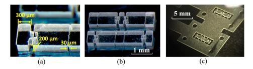
Figure 3. Optical micrographs of (a) the 200- $\mu$ m-thick SU-8 structures (rigid half-scissor linkages for active alignment) with 30- $\mu$ m microfabricated gaps for hinge bending; (b) the upper and lower hinge structures implemented in SU-8 for an actively aligned 3 mm  $\times$  0.67 mm microscissor; and (c) the 200- $\mu$ m-thick SU-8 structures tethered on the supporting alignment frames for the passively aligned assembly.
