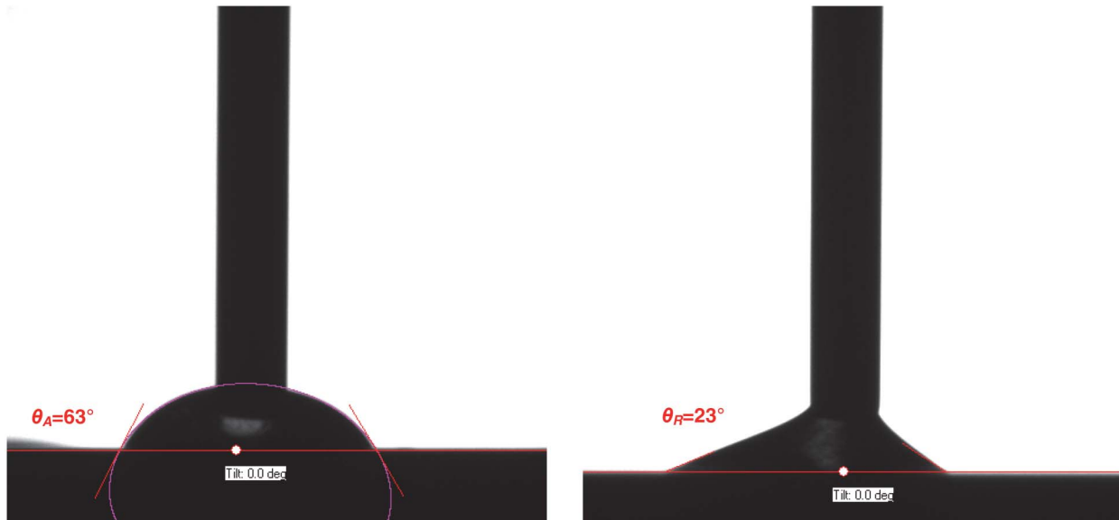
Fig. 16 Static advancing contact angle (left) and static receding contact angle (right) on the heavily oxidized heater surface
