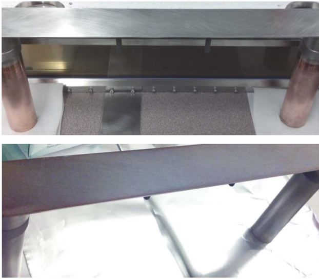
Fig. 3 Photograph of nominal plate (top) and plate following 600°C oxidation in air (bottom)
