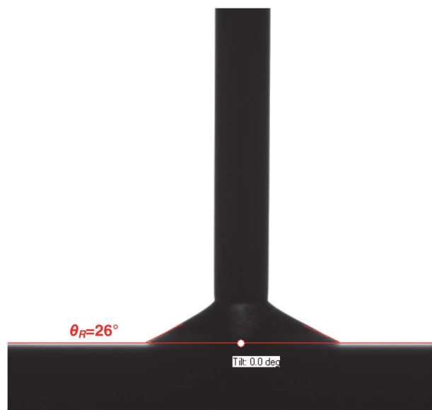
Fig. 14 Static advancing contact angle (left) and static receding contact angle (right) on the nominal heater surface
