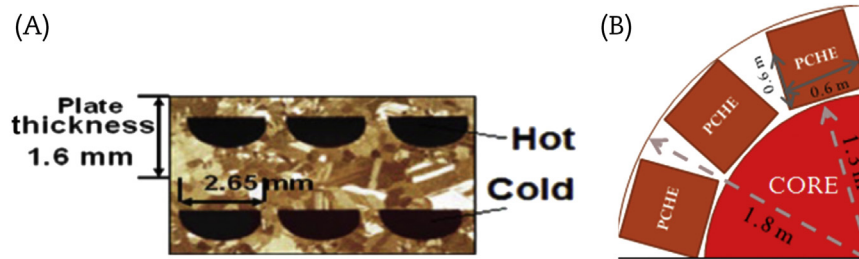
Fig. 1 – (A) Cross-section of two layers of the printed circuit heat exchanger (PCHE) showing the semicircular coolant paths [21]. (B) The 1/4 layout of the PCHE in the vessel relative to the core (it is noted that the core is at lower elevation compared to the PCHEs).
