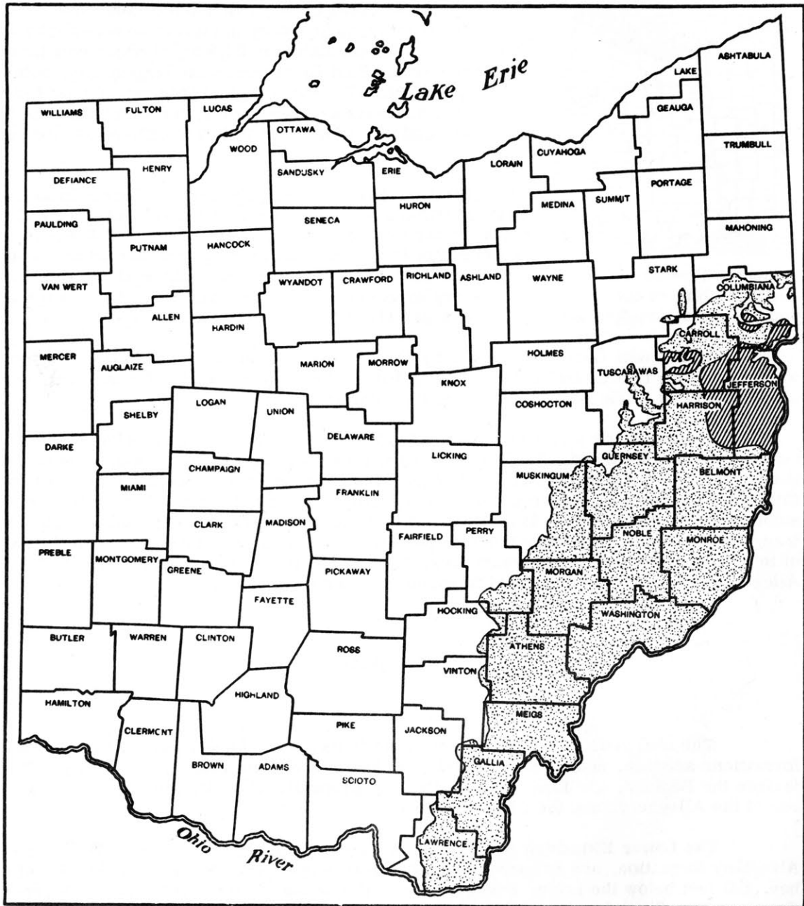
Figure 13 - Area underlain by the Lower Freeport (No. 6a) coal bed of the Allegheny formation in Ohio. Diagonal pattern, area of estimated reserve; stippled pattern, area of other Lower Freeport coal.
