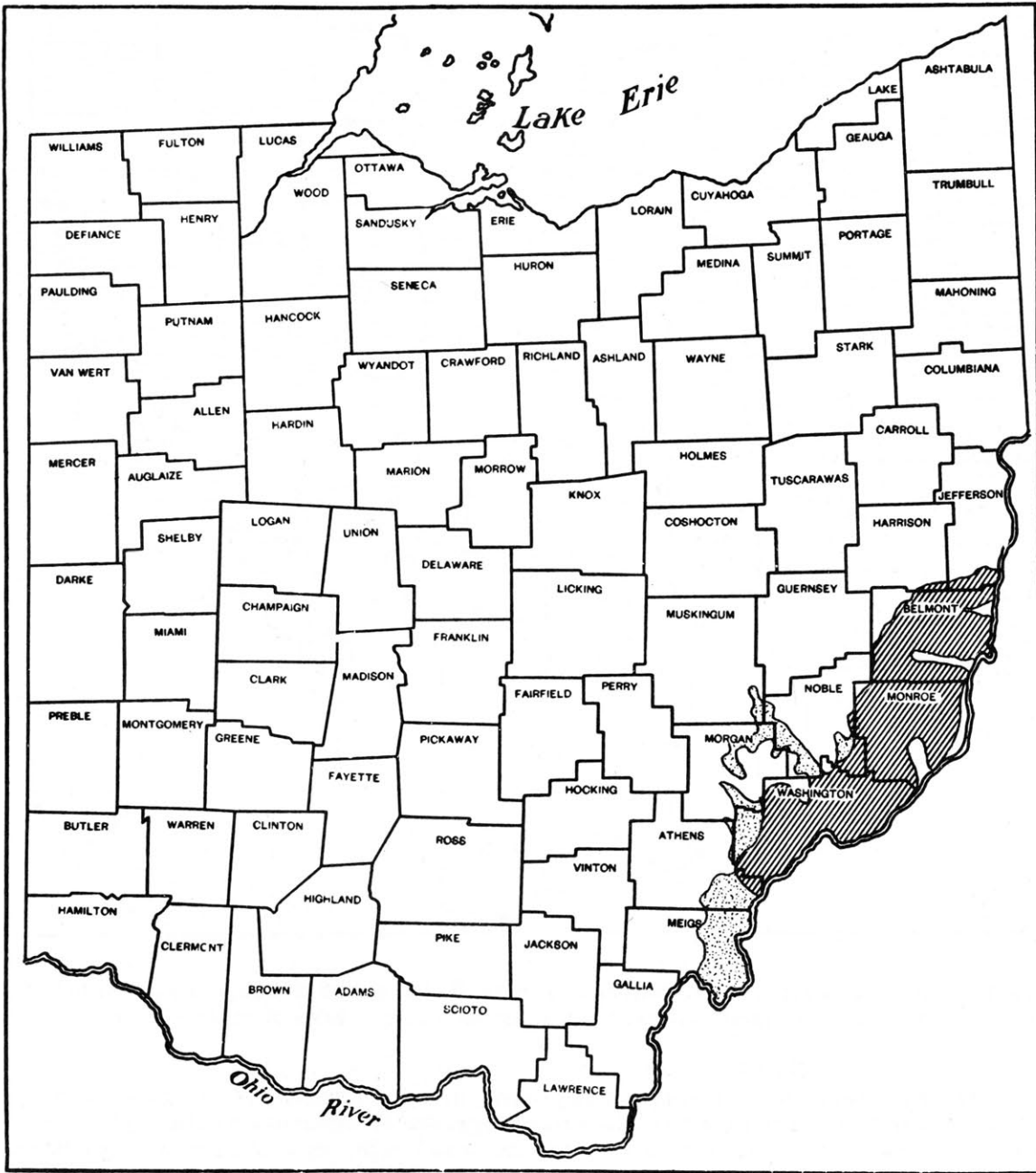
Figure 21 - Area underlain by the Uniontown (No. 10) coal bed in Ohio. Diagonal pattern, area of minable coal; stippled pattern, area of other Uniontown coal.
