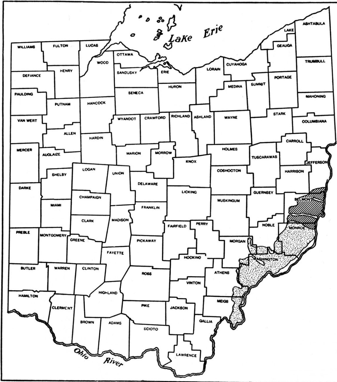
Figure 22 - Area underlain by the Waynesburg (No. 11) coal bed in Ohio. Diagonal pattern, area of estimated coal reserve; stippled pattern, area of other Waynesburg coal.
