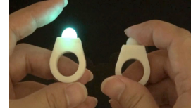
Figure 1: Squeezing the ring to send a lighting and a vibro-tactile signal to the paired partner.
