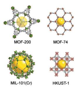
**Figure 13.** Representative types of MOF structures which exhibit high gas storage properties. MOF-200: H<sub>2</sub>; MOF-74: CO<sub>2</sub>, NO, CH<sub>4</sub>; MIL-101(Cr): H<sub>2</sub>, CO<sub>2</sub>; HKUST-1: CO<sub>2</sub>, NO, CH<sub>4</sub>.
