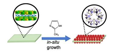
**Figure 17.** In situ growth of ZIF-8 nanocrystals on Zn–Al–LDH. (Colour scheme: Zn, purple; C, black;  $H_2O$ , blue spheres;  $A^{n-}$ , cyan spheres). Adapted from *Dalton Trans.* **2016**, *45*, 12632–12635. Copyright (2016) Royal Society of Chemistry.
