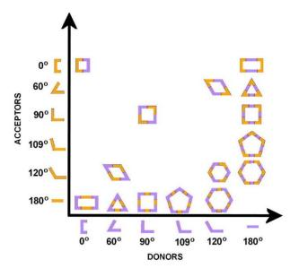
**Figure 19.** Formation of 2D architectures constructed by self-assembly of ditopic building blocks. Adapted from *Chem. Rev.* **2011**, *111*, 6810–6918. Copyright (2011) Royal Society of Chemistry.
