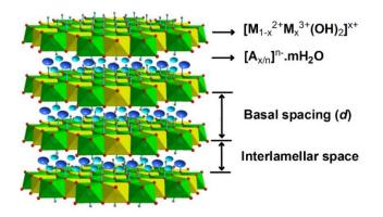
Figure 16. Schematic representation of the classical LDHs structure [88]. Adapted from Catalysts 2017, 7, 260.
