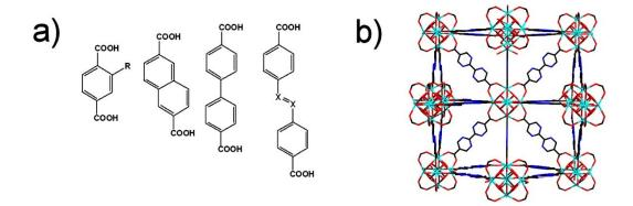
**Figure 15.** Structure of the organic linkers used in the MOF synthesis (**a**), and the structure of Zr-L<sub>6</sub> MOF (**b**). (Colour scheme: Zn, cyan; O, red; C, black; N, blue).
