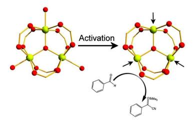
**Figure 14.** The coordinated water molecules are removed from MIL-101(Cr) generating free coordination sites (highlighted with black arrows) during the activation process. Subsequently, the activated MIL-101(Cr) catalyses the cyanosilylation of benzaldehyde. (Colour scheme: Fe, lime green; O, red).
