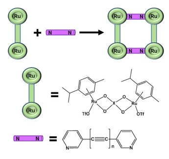
Figure 22. Self-assembly of tetranuclear molecular rectangles.
