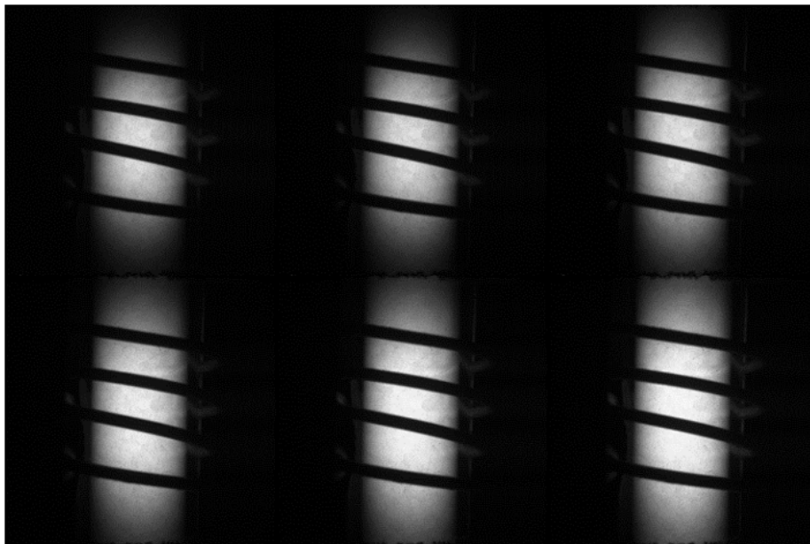
FIGURE 4.34: Top 100 W, 150 W and 200 W. Bottom 250 W, 300 W and 350 W. Photographed light intensity variation of Ar H-mode plasma as a function of power.
