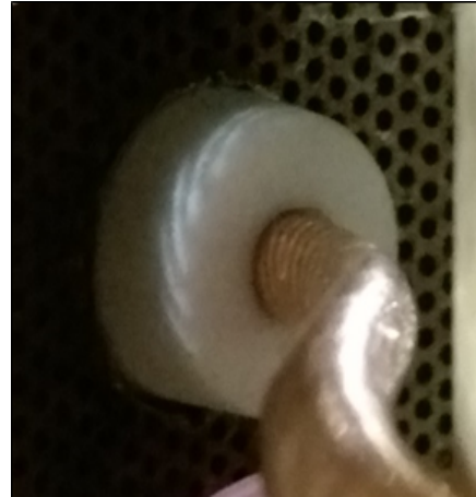
(B) Photograph of teflon insulation used to prevent breakdown between the inductive coil and Faraday Cage
