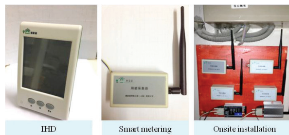
Fig 2. Real images of IHD, smart meter and onsite installation
