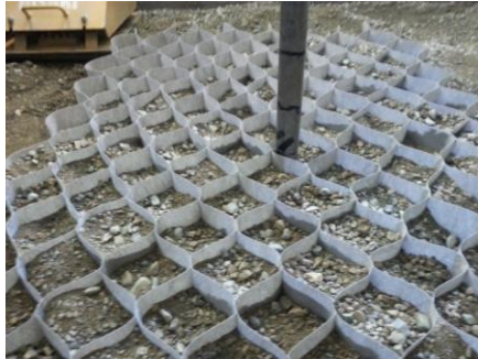
Fig. 2. A view of geocell (TDP Limited) spread over anchor plate in the test pit.
