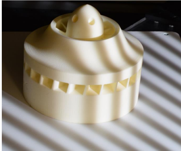
Figure 1. A sinusoidal fringe pattern projected onto a polymer AM part from the bottom right hand corner of the image. The irradiance distribution across the part is used to reconstruct the surface.
