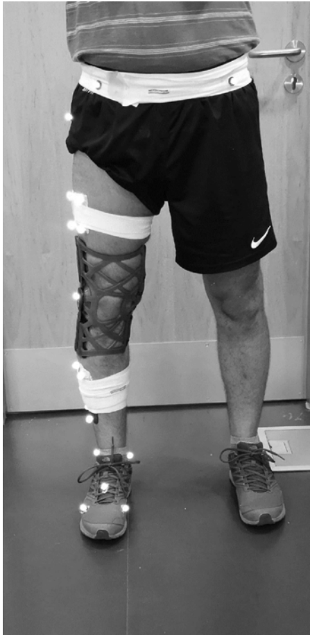
Figure 1: Retroreflective marker set with the proprioceptive knee brace (OA Reaction, DJO, USA).
