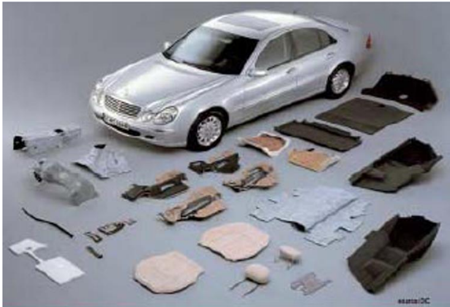
Figure 1.1 Applications of natural fibres reinforced composites in a Mercedes E-class, image adopted from (JEC Magazine, 2009).
