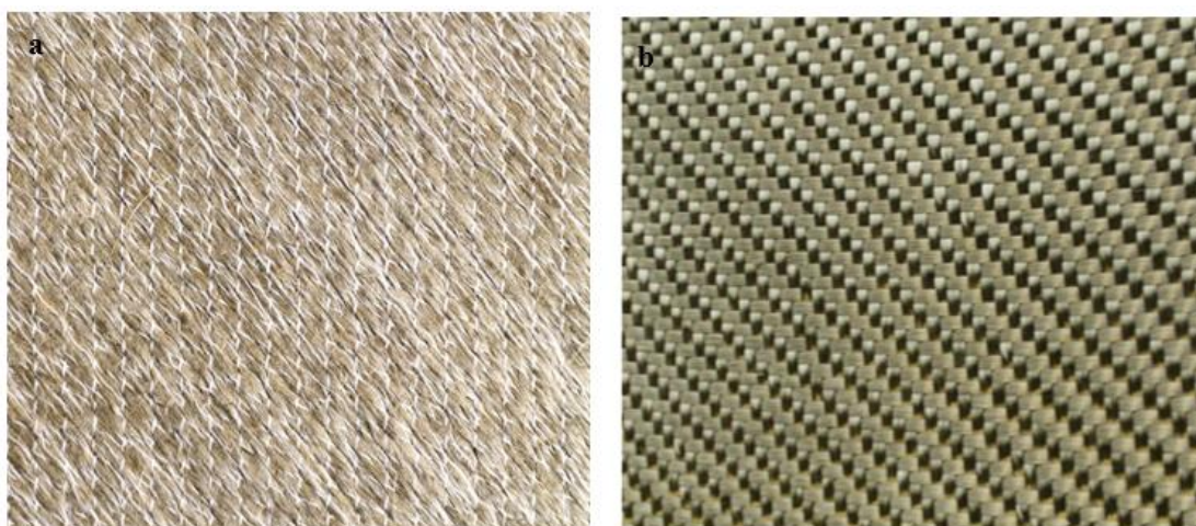
Figure 3.2 Reinforcement fibers a) Biotex flax \pm 45^\circ biaxial fabric 600 \text{ g/m}^2 b) Basalt multiaxial fabric BAS BI 600 \text{ g/m}^2 (BASALTEX 2016; Composites Evolution 2012).
