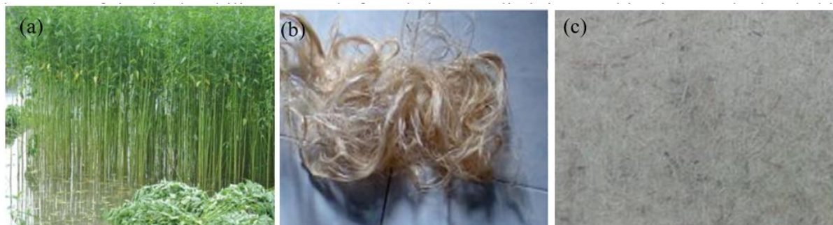
Figure 2.10 Kenaf plant (Ramesh et al. 2017), (b) kenaf fibre (Satyanarayana et al. 2009), (c) non-woven kenaf fabric mat (Sharba et al. 2016).
