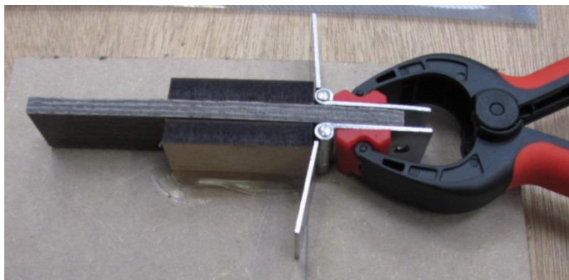
Figure 3.13 Using C-clamp to attach the hinges for DCB specimens.
