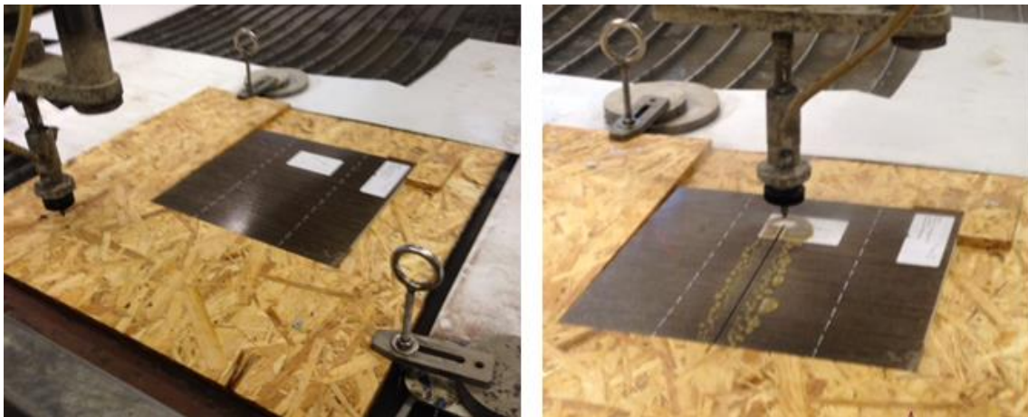
Figure 3.11 The water jet cutting process of FVE panels.
