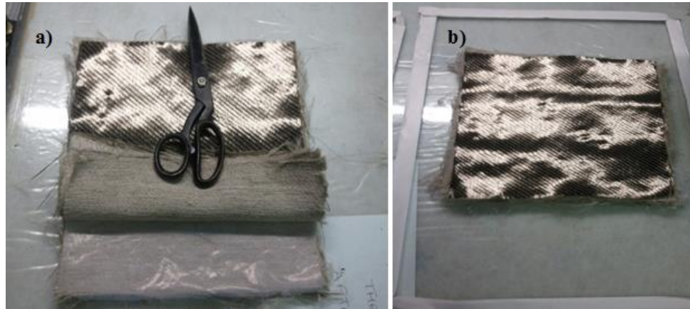
Figure 3.5 Woven Biaxial Fabrics: a) four layers of flax balanced, with one layer of PTFE \mu\text{m} in the middle; b) Six dry layers of flax on a glass plate.
