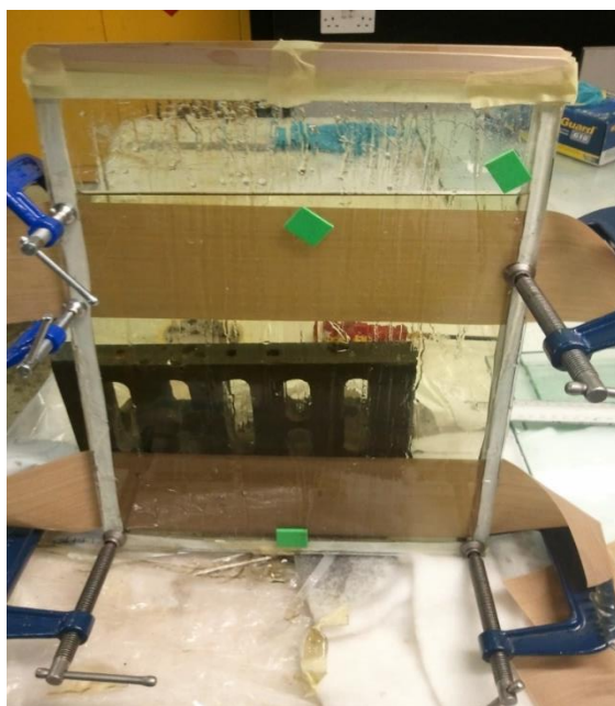
Figure 3.9 Vertical casting process of neat VE.
