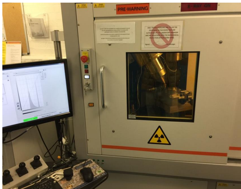
Figure 3.24 image of \mu CT machine of Nikon (Xtec) XT H 225.
