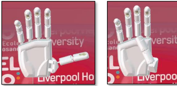
Figure 3. Thumb extension and flexion.
