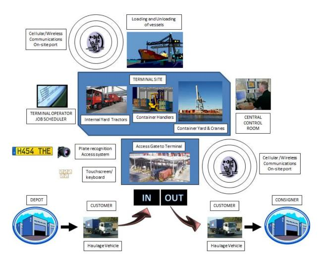
Figure 1. Depiction of ICT solutions comprising the structure of seaport terminals investigated in this research work.
