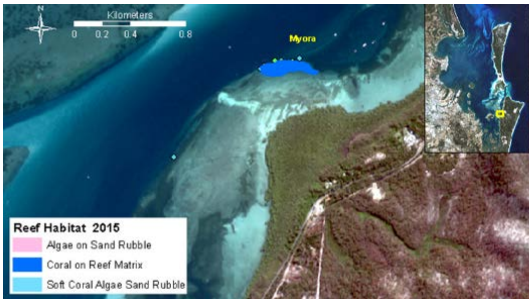
Figure 11: Myora reefal areas, derived through manual digitisation guided by 2014 ZY-3 satellite image (5 m x 5 m pixel) as a backdrop overlaid with spot check field data for interpretation.
