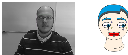
Fig. 1. A robotic head Flobi (simulated) imitates the facial expression of a human in front of a web cam. The green rectangle on the left marks the input image determined by a face detector. Motor values (perc.) for each actuator are given at the respective joints.
