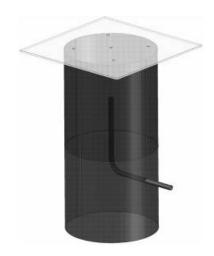
Tube 4: used for cultivation of microbial mats in the laboratory and in the Lake Room of Movile Cave. The length of the polypropylene tube is 220 mm, its inner diameter 105 mm. The quadratic lid on top consisted of either glass (anoxic atmosphere the tube) or perforated Plexiglas. In anoxic tubes, a polyvinyl chloride hose allowed the bubbling out of surplus methane out-gassing from the hydrothermal water into the tube (see text).
