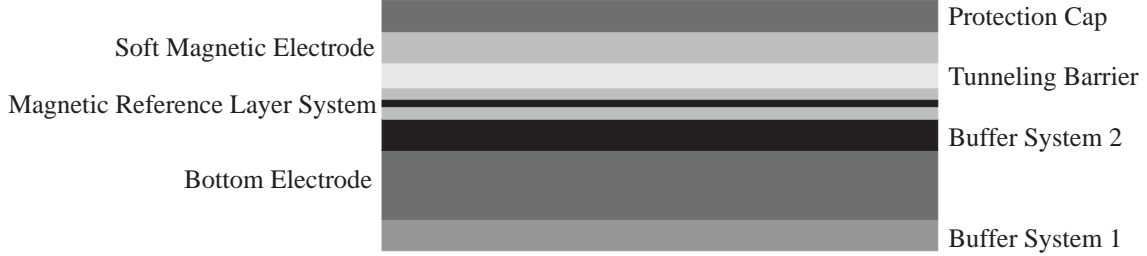
Figure 2.7: Sketch of a standard spin dependent tunneling stack. The different functional groups drawn may consist of sub–groups. The thicknesses correspond not to a real system.
