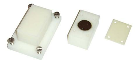
Figure 4.14: Sample stage for usage in the TMR measurement place, provided by MONIKA BRZESKA. The cubic nylon block in the middle contains one permanent magnet for PPD measurements, and is capped with the nylon sheet on the right side. Measurements without an out-of-plane field are done with the massive nylon block on the left side.
