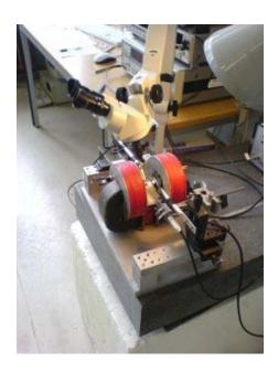
Figure 2.6: TMR measurements setup.
