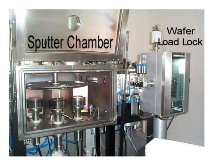
**Figure 2.1:** CLAB 600 – main chamber and load lock. (Taken from "D2 – lab tour" at www.spinelectronics.de.)
