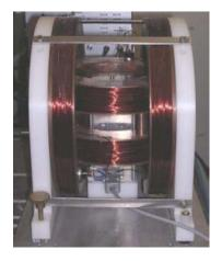
Figure 4.8: Setup with two pairs of Helmholtz-coils by JÖRG SCHOTTER. [Sch04, figure 14]
