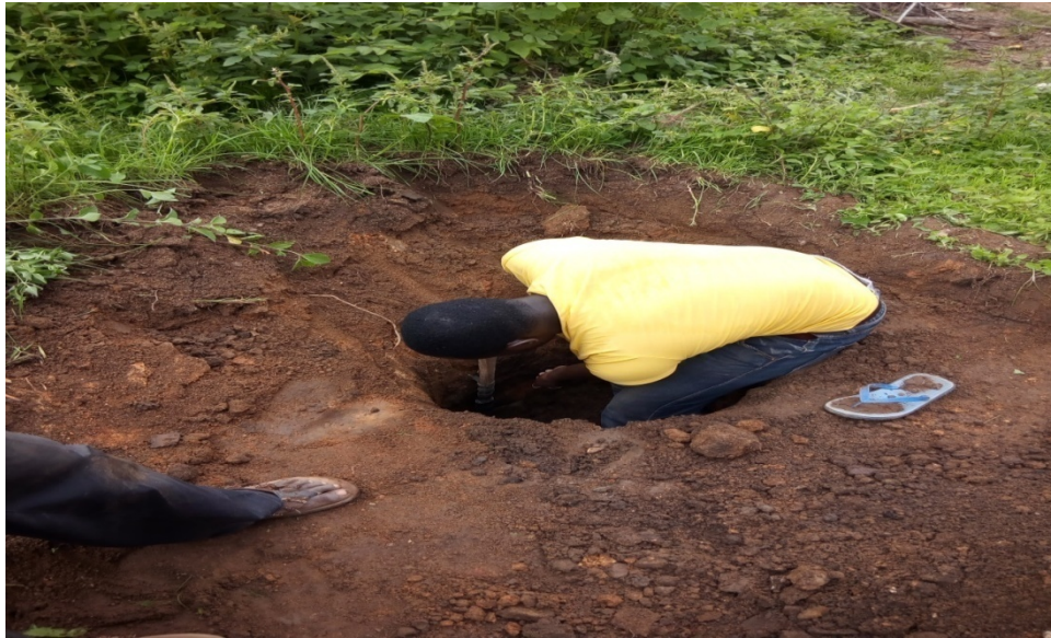
Plate 1. Overburden Removal in Lotto Mining
