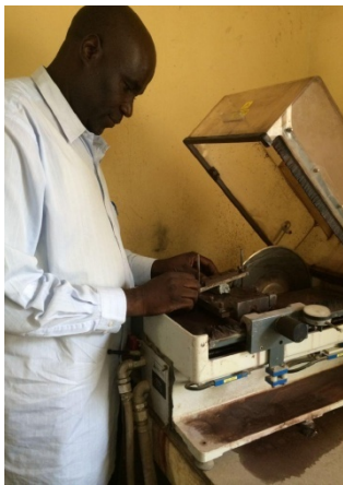
Figure 1. Alogitech GTS 1 Thin Section Cut Off Saw
