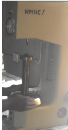
Figure 3. Rockwell hardness testing machine
