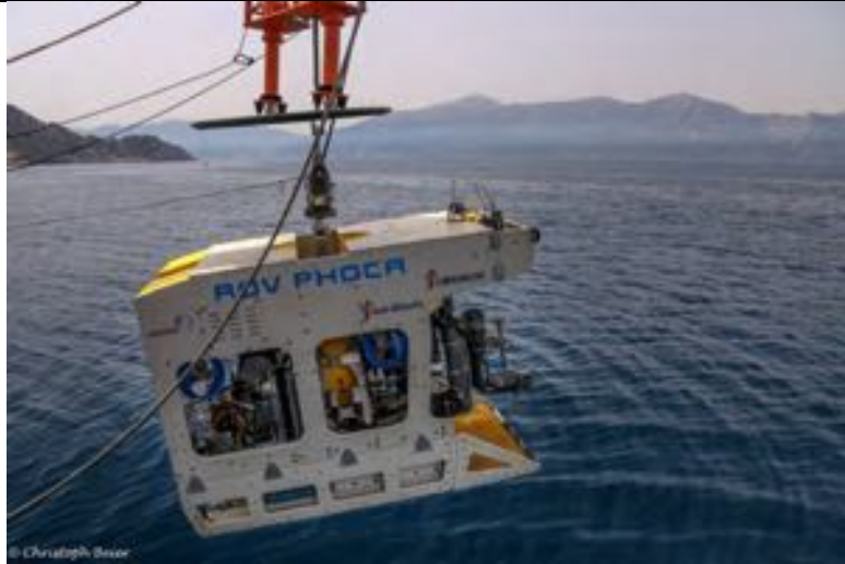
Figure 2. ROV PHOCA being launched from RV Poseidon in the Epidavros Basin during POS512
