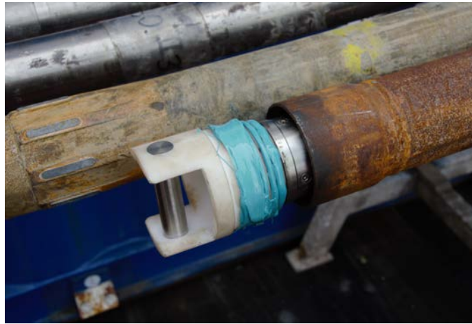
Fig. 45: Picture of the system on board MERIAN prepared with fresh sealing to be mounted on an iron drill string.
