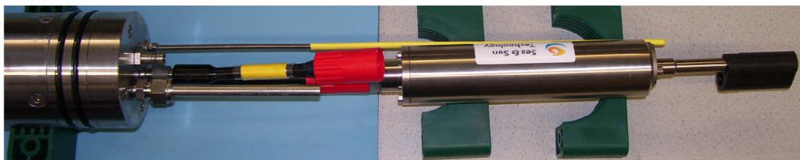
Fig. 44: MeBoPlug prior to being screwed into a MeBo drill pipe (left); right photograph shows bottom view into the borehole with ports for P (hole at left) and T (little pin at right) monitoring. See text.
