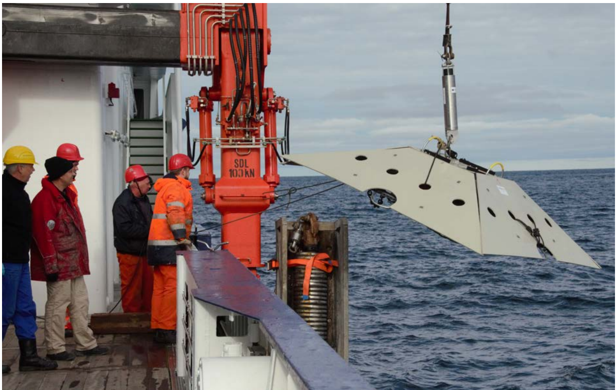
Fig. 49: Sonar-CORK deployment handling on board R/V MARIA S. MERIAN.
