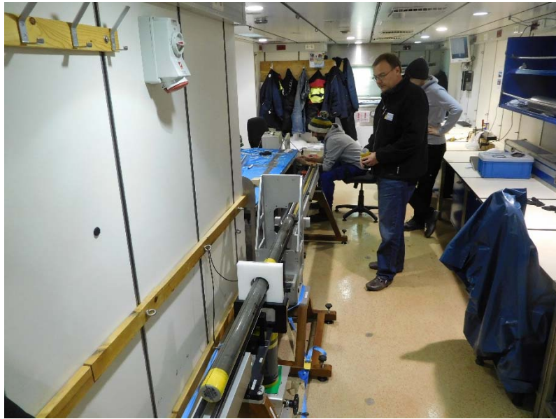
Fig. 69: Logger with smaller-diameter loop (6.5 cm) to log MeBo cores, available for Leg 2 of MSM57 only.
