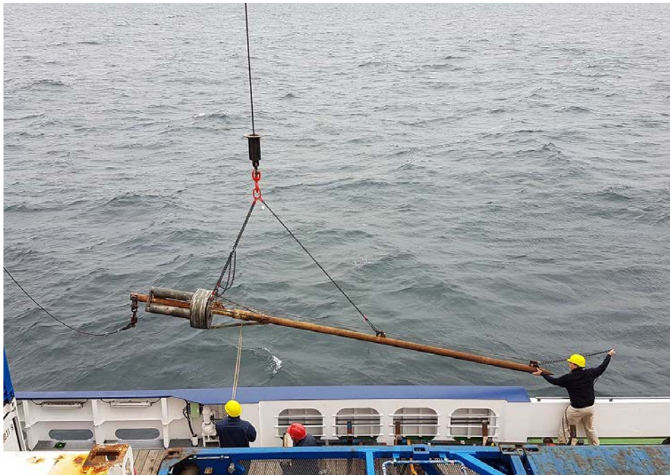
Fig. 25: Image of the deployment of the temperature probe on August 2 nd at the starboard side of R/V MARIA S. MERIAN.
