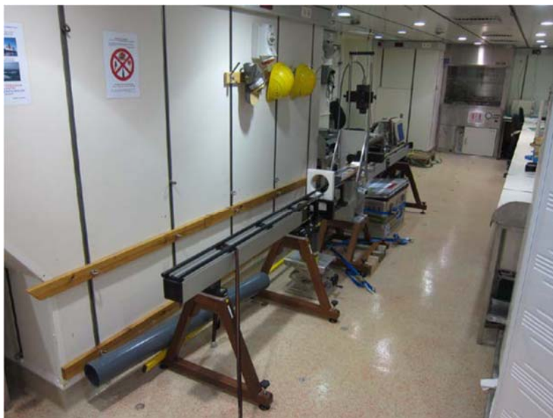
Fig. 68: Logger with large-diameter loop (14 cm) to log gravity cores.
