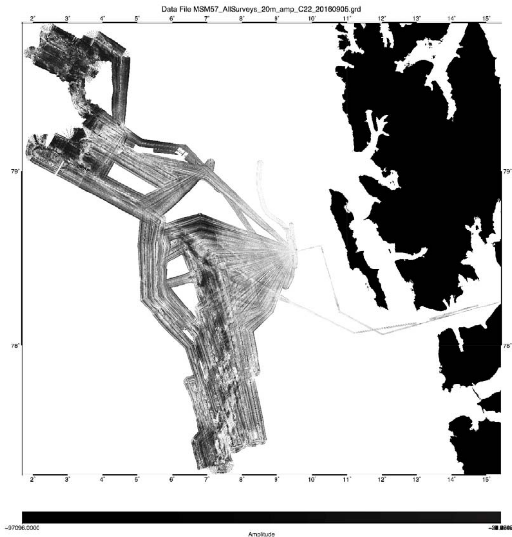
Fig. 21: Amplitude map of MSM57 (Leg 1 and 2) using 20 a meters' resolution. Bright values show a strong backscatter amplitude.
