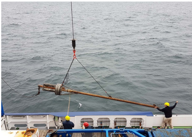
Fig. 4: Heat flow lance from GEOMAR during its deployment during Cruise MSM57.
