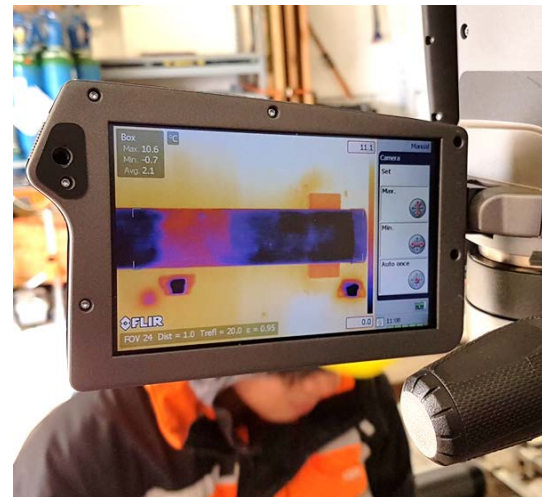
Fig. 63: Left: The infrared camera was fixed on a tripod with a focal distance 150 cm between camera and core liner. Ice cubes were used as reference position for post processing and stitching of the images. Right: The monitor of camera shows the temperature anomalies simultaneously while scanning of GC-9. The cold region (dark blue to black) indicated the appearances of gas hydrate, the warm part (red to orange) indicated the voids in the core liner.
