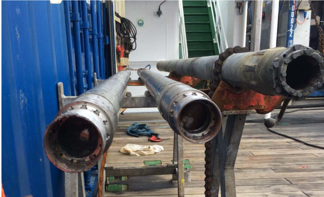
Fig. 95: Sealed bottom valve of MDPs deployed at station GeoB21613-1 (cores 29P and 30P).
