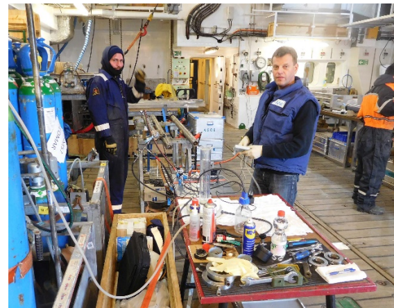
Fig. 5: Degassing of the autoclave core barrel (MDP) retrieved from MeBo drill site.
