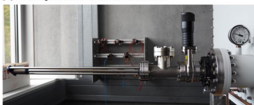
Figure 4.2: (a) Transportable vacuum chamber to transfer samples between glovebox and integrated UHV-cluster under vacuum or inert gas. This transport box is equipped with a DN 40 ISO-KF flange that allows easy and fast handling. (b) Airtight XRD sample holder. The dome is screw tightened with a special tool inside the glovebox.
