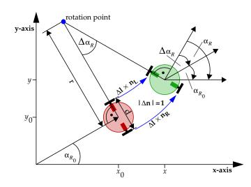
**Figure 4.** Graphical representation of the position calculation by path integration showing the current and the previous position.
