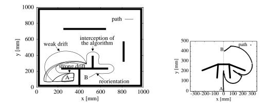
**Figure 17.** Trajectory of the robot during the A-to-B-navigation process in a simulated (left) and a real (right) environment.
