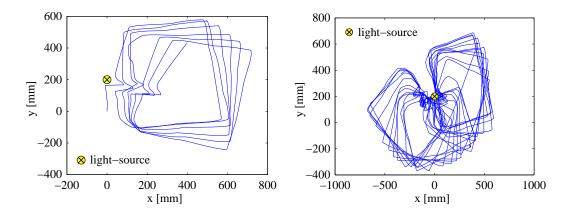
**Figure 33.** Path of the real Khepera in two experiments for the position adjustment with one singular light source in an area of  $75 \times 60$  cm.
