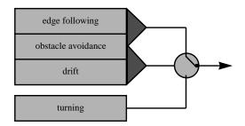
**Figure 6.** The interaction structure incorporating both the basic schemata responsible for the exploration of an unknown environment (without drift schema) as well as the point-to-point navigation to a destination of known position (including the drift schema).
