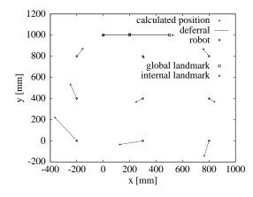
Figure 40. The error which occurs during recording the landmarks' positions (solid line) prevents an exact calculation of the robot's position.
