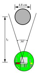
Figure 25. Schematic illustrating the recognition of a cylinder as a landmark using the linear camera.
