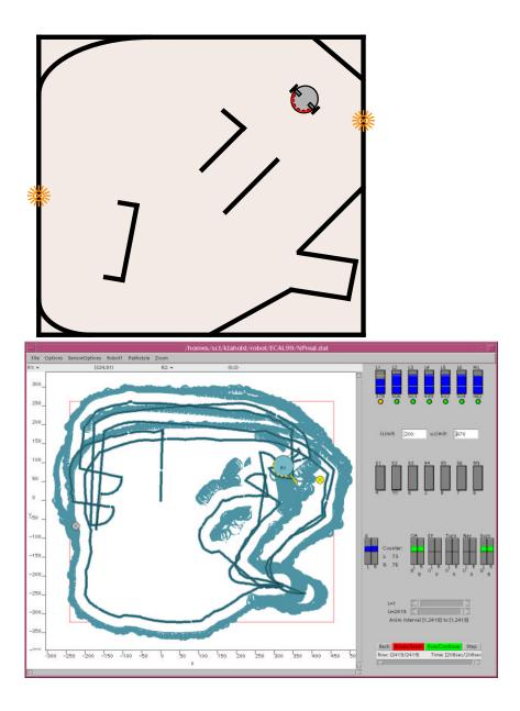
**Figure 42.** Visualization (bottom) of a complete data set recorded from a real experiment concerning the Dynamical Nightwatch's Problem together with the corresponding environment ( $80 \times 80 \text{ cm}$ ; top). Note the drift of the internal position.
