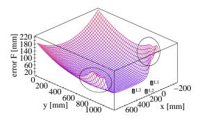
**Figure 39.** Error (Eqn. 45) due to inaccuracies during the measurement of the angles in dependence of the robot's position.
