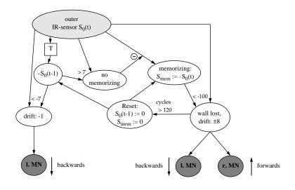
**Figure 12.** Neural interpretation of the edge following algorithm (the wall is assumed to be on the left side of the robot; I./r. MN  $\triangleq$  left-/right motor neuron).
