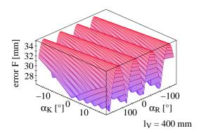
**Figure 36.** Graph of the error (F) (Eqn. 32) which occurs during the calculation of the landmark's position in dependence of the position of the landmark in the picture ( $\alpha_K$ ) and the angular orientation of the robot ( $\alpha_R$ ).
