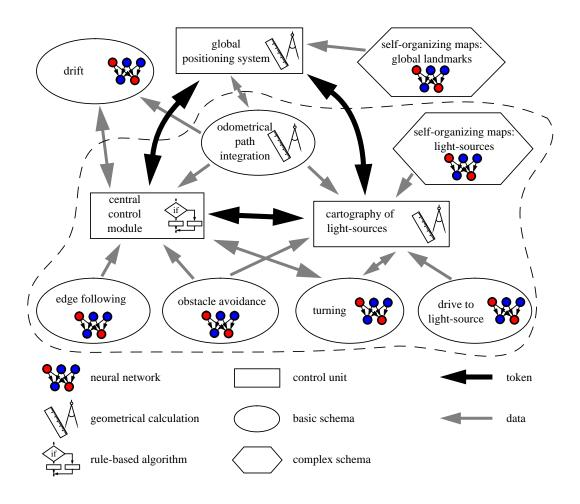
**Figure 41.** Representation of the interaction schema that realizes a solution to the Foraging Animate Problem.
