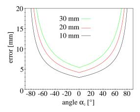
Figure 31. The three curves display the error (Eqn. 28) which occurs at three different distances to the light-source (10 mm, 20 mm, 30 mm).
