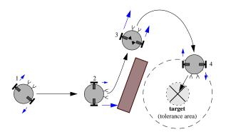
Figure 14. Example of a navigation sequence.
