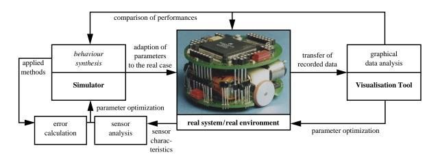
Figure 3. The design cycle. Essential to the proposed concept is the close coupling between behaviour synthesis and various analysis loops.
