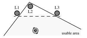
**Figure 34.** Margins of the area in which the Khepera is able to recognize the landmarks (L1-L3) correctly.
