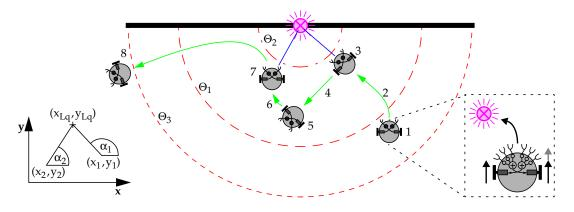
**Figure 29.** Mapping sequence of a light-source. The areas marked by the thresholds  $\Theta_1$ - $\Theta_2$  correspond to the dashed lines in Fig. 19.
