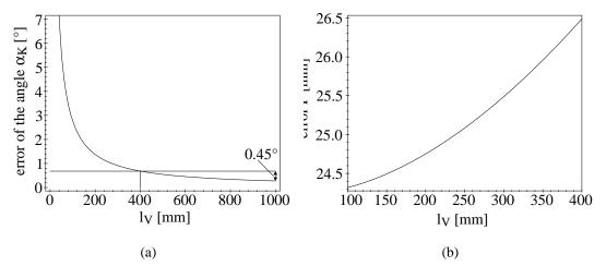
**Figure 35.** The corrected error vs. distance from the landmark (a) and the Graph of the error (F) (Eqn. 32) which occurs during the calculation of the landmark's position vs. the distance (l) to the landmark  $(\alpha_K = 0^\circ, \alpha_R = 0^\circ)$  (b).
