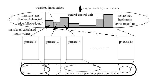
Figure 2. Schematic of the implementation concept, which assures the efficient usage of the given system resources.
