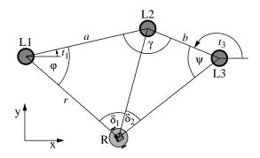
**Figure 37.** Schematic for the calculation of the robot's position (R) by means of the three landmarks (L1 - L3).
