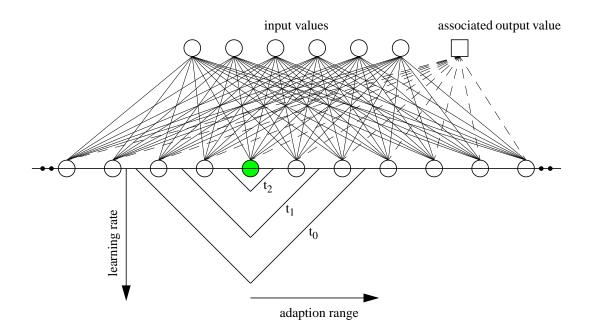
**Figure 18.** Schematic of a 1-dimensional self organising map (SOM) during the training period.
