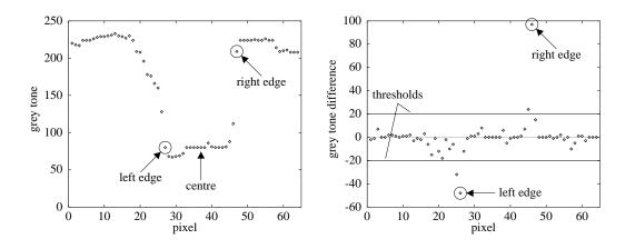
**Figure 26.** Picture of a landmark in view of the robot as sub-symbolic vision data (left) and the resulting gradient picture (right).
