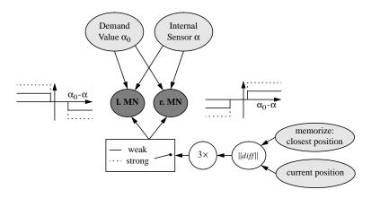
Figure 15. Neural structure that implements the drift (Fig. 13) as well as the turning schemata (Fig. 16).
