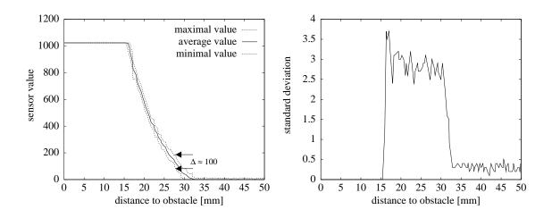
**Figure 7.** The distance characteristic (left) of the infrared sensors on the robot (sensor  $S_2$ , middle left) and the corresponding standard deviation (right), whereby the mean value has been taken from 50 samples.
