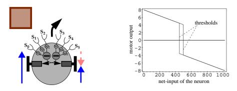
**Figure 10.** Representation of the neural network that implements the obstacle avoidance behaviour (left) with the activation function of the neurons (right).
