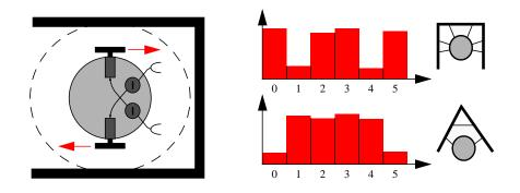
**Figure 16.** If it is not possible to leave a pre-defined circle during a given number of program cycles (left) or if its front IR-sensors perceive certain characteristical patterns (right), the robot performs a  $180^{\circ}$  turn.
