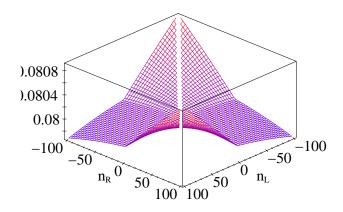
**Figure 5.** Arising position errors per program update cycle due to noncontrollable influences, in particular slippage, during the process of odometrical path integration.
