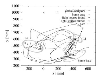
**Figure 44.** Trajectory of a real Khepera in an unknown environment with two light-sources (L1, L2) and a home-base (the ellipses mark the areas in which the respective object has been recognized).
