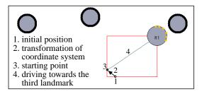
Figure 43. Visualization of the initial landmark mapping in a real experiment.
