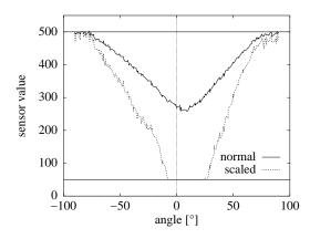
**Figure 22.** Set of values from sensor  $S_3$  in a quadruplicate distance to the light-source with respect to the one the SOM was trained with.
