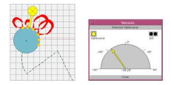
Figure 24. Visualization of the trained neural network for the light-sensor calibration.
