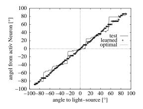
**Figure 23.** Result of the training, showing the test of the neural network with the data set used for learning (fat dotted line) and respectively with a data set resulting from a quadruplicate distance to the light-source (thin solid line). As reference a straight line is drawn. In spite of the scaling, a large distance sensitivity may be recognized.
