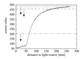
Figure 19. Characteristic curve of the light-sensors.
