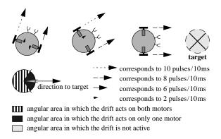
Figure 13. Representation of the effects of the drift schema depending on the angular miss-alignment.
