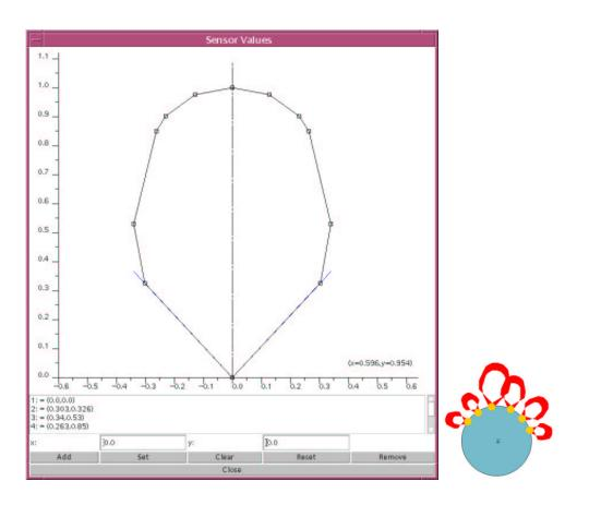
**Figure 8.** The scalar sensor values are—by means of the adjustable angular characteristics (left)—transformed to areas in which an obstacle may be located (right).
