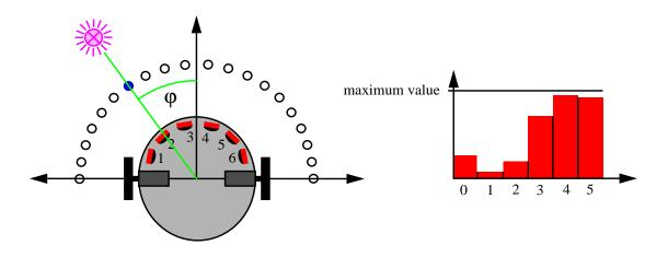
**Figure 20.** Schematic of a 1-dimensional self-organizing neural network which is used to extract a symbolic angle-to-light-source information (left) from the sub-symbolic sensor stream (right). Note that the sensor values are inverted (Fig. 19).
