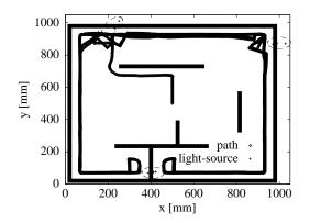
Figure 32. Path of the simulated Khepera which always recognized the three different light-sources correctly.
