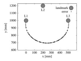
**Figure 38.** The diagram shows the positions at which a calculation of the position is impossible assuming given locations of the landmarks.
