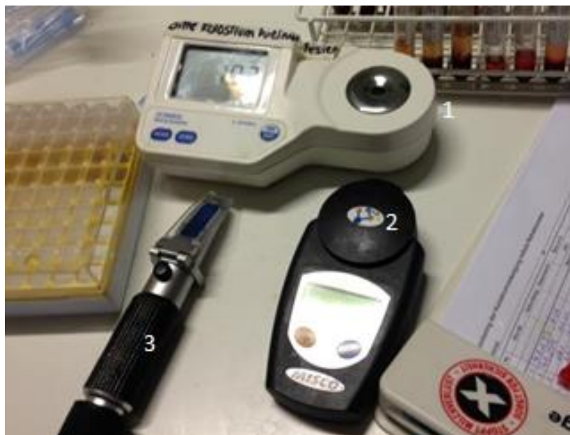
Figure 5. Devices used in the study; 1) Device 1: Digital refractometer Hanna HI 96801; 2) Device 2: Digital refractometer Misco PA201; 3) Device 3: Optical refractometer.
