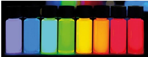
Figure 1.8: When they are excited by ultraviolet light (pictured), colloidal quantum dots fluoresce at different colors depending on the particle size.
