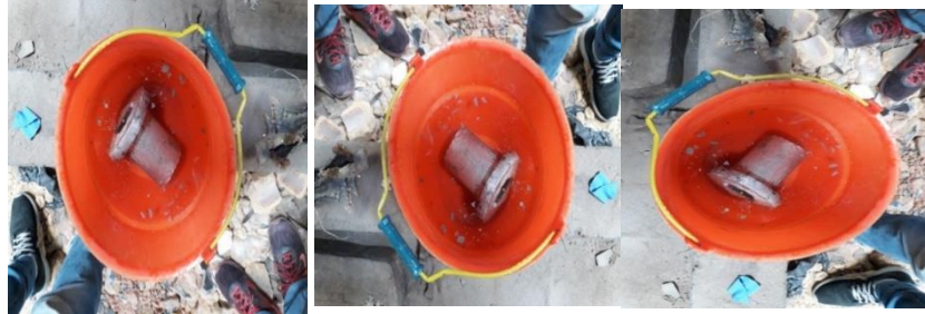
Gambar 6. (A)Media pendinginan air suhu 15°C, (B) Media pendinginan air suhu 27°C, (C) Media pendinginan air suhu 55°C.
