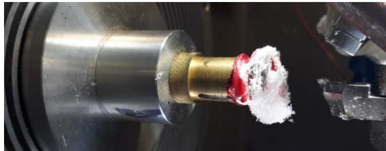
Figure 76: Observation 14 chip build up.
