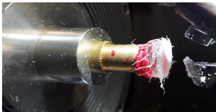
Figure 60: Observation 5 chip build up.
