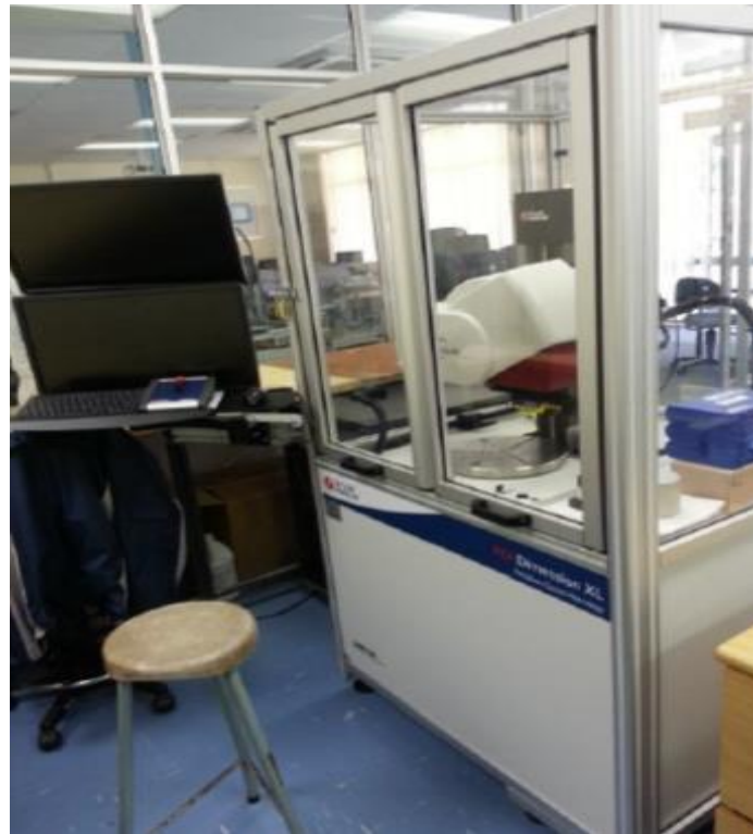
Figure 32: Taylor Hobson PGI Dimension XL surface profilometer at the Precision Engineering Laboratory, Nelson Mandela Metropolitan University.
