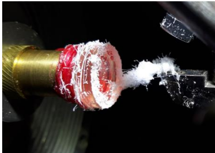
Figure 64: Observation 14 chip build up.
