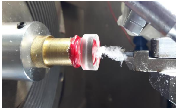
Figure 72: Observation 4 chip build up.
