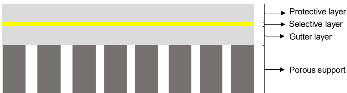
Figure 11. Schematic illustration of a usual thin film composite membrane used for industrial gas separations.
