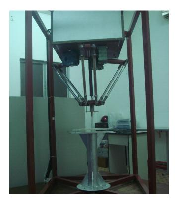
Fig.3. Delta parallel robot for experiments.
