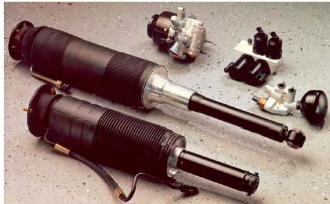
Figure 1-3 Mercedes-Benz C Class Active Body Control Actuators,[9]
