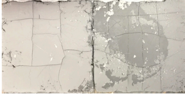
Figure 70: Frosted sample after 10 thermal cycles
