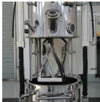
Figure 23: Side view of DPM tank and agitators
