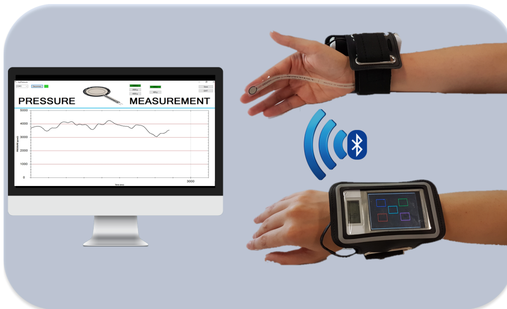
Figure 1. Instrument to monitor and register the pressure
