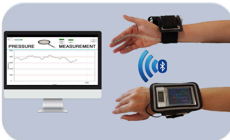
Figure 1. Instrument to monitor and register the pressure
