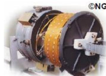
Figura 10 - Mastro Coilable (T. Murphey ,2008).
