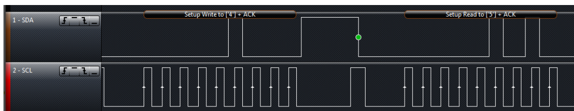
Figure 4.17: Testing I^2C communication using a Explorer 16 and an Arduino.
