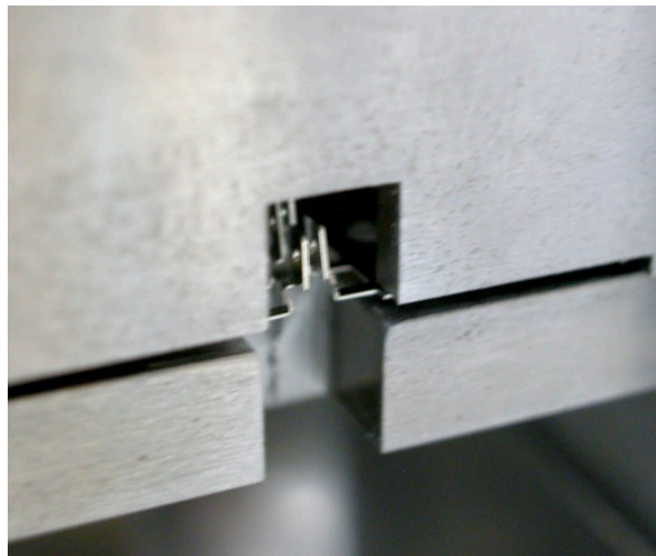
Figure A.10 Holding the contact spring assembly in the cutting tool after separating it from the lead frame
