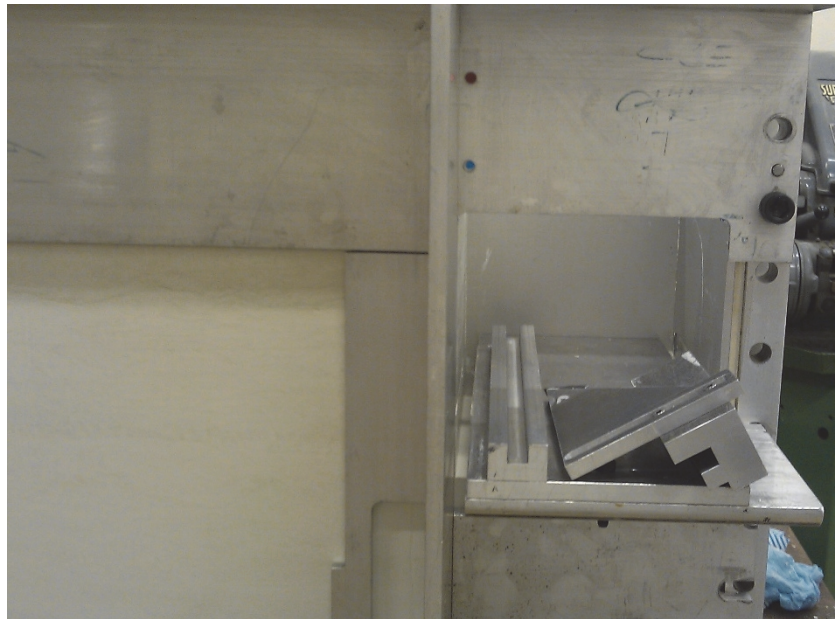
Figure 5. 40 Guide and cutter for forming the 40 mm deep slot for the model wall toe embedment.
