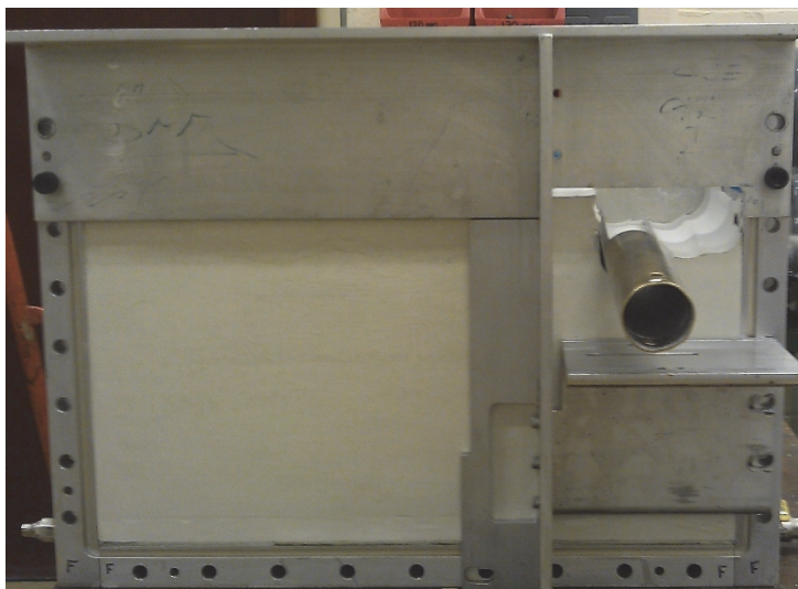
Figure 5. 39 Photograph showing the excavation trimming guide being used to rough cut the excavation cavity using the brass tube cutter.
